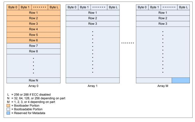
The following diagram shows the device's flash memory layout for the PSoC 3 and PSoC 5.
