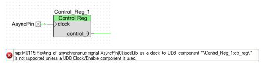
As stated in the error message, the error can be removed by using a UDBClkEn component in async mode. That won't remove the underlying synchronization issue, but it will allow the design to override the error if the design has handled synchronization in some other way.
