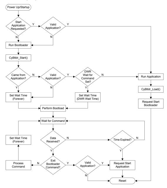
The following diagram shows how the bootloader works.
